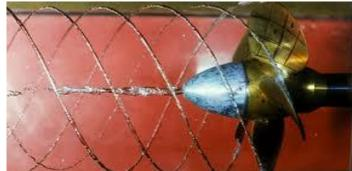
Execution of tests in the Froude's channel for the determination of the resistance of models of ships mono-hulls and multi-hulls. Execution of propellers' tests in the Cavitation Tunnel.
